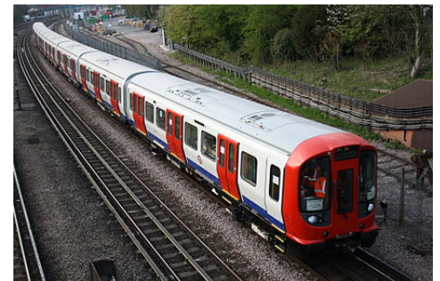
The S7/8 Stock on the London Underground can return around 20% of its energy usage to the power supply. [1]
