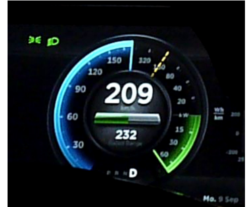
A Tesla Model S P85+ using regenerative braking power in excess of 60 kW. During regenerative braking the power indicator is green
